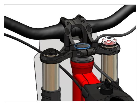
If your bike is experiencing this issue, please contact OSET to source an additional 2mm headset spacer, which when installed beneath the headset top cap, allows the system to be tightened correctly.
