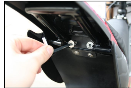
(1.) Unscrew & remove seat bolts.
