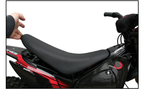
(2.) Lift seat up & forwards to release.
