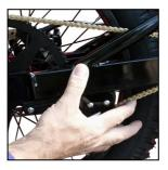
These two pictures show the correct tension. When pushing up on the chain, it should only move between 5 and 10mm.
