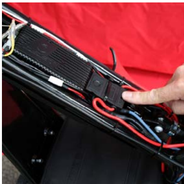
Controller and fuse.
